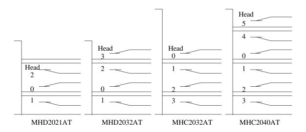
Figure 2.2 Configuration of disk media heads
